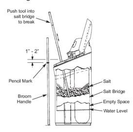
Carefully push into the bridge in several places to break it. Do not try to break the salt bridge by pounding on the outside of the salt tank. You may damage the tank.
